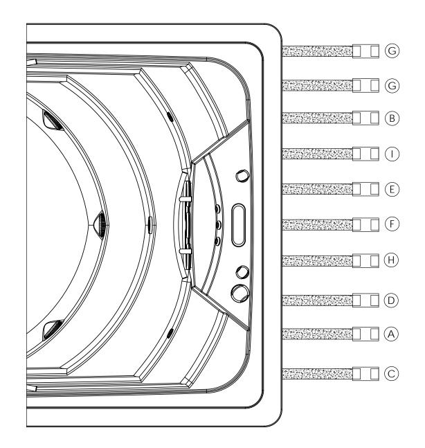
(\*) Massage Pump can be installed on each Massage Circuits specified, depending on the layout of the installation
